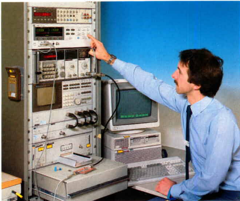
Incoming inspection of RF devices using the HP 8508A
